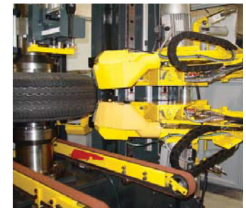
Optional Center Grinder (above) and Shoulder Grinders (below) provide for tire optimization and higher yield
