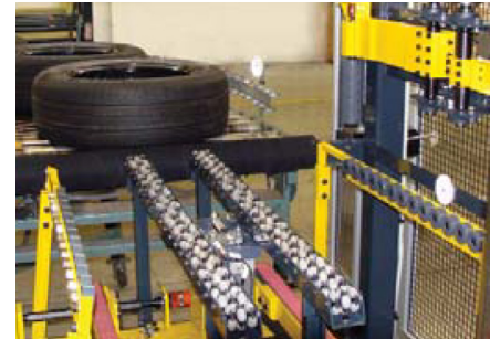
Handler & Luber with automatic adjusting tire centering
