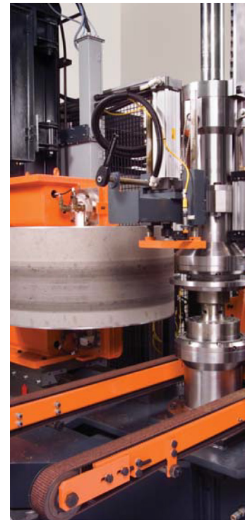
Loadwheel and tooling is easily accessible for tooling change and maintenance
