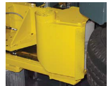
Optional Center Grinder (above) and Shoulder Grinders (below) provide for tire optimization and higher yield
